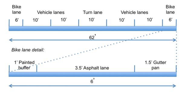
Current WCRC policy is to make all vehicle lanes at least 11'. This often makes sense, especially on high-speed 2-lane roads. But in a more urban setting like Packard, the above lane configuration would improve safety for all road users because:
